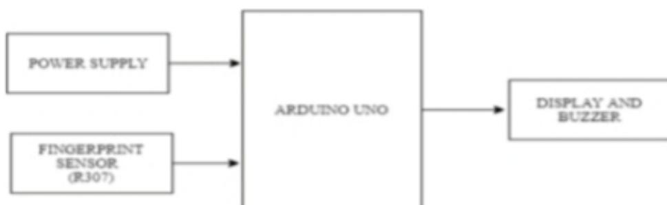
Figure 3.1 Block diagram of verification unit
