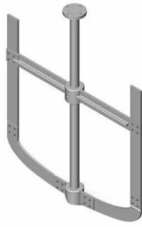
Fig.2: Pictorial figure of Anchor Agitator
