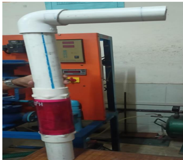
Fig.9. Waste PVC pipe for full distillation column
