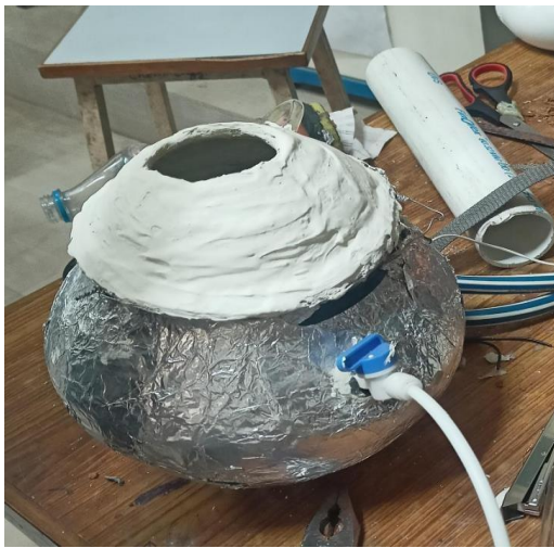
Fig.6. Earthen pot with inbuilt heater for reboiler
