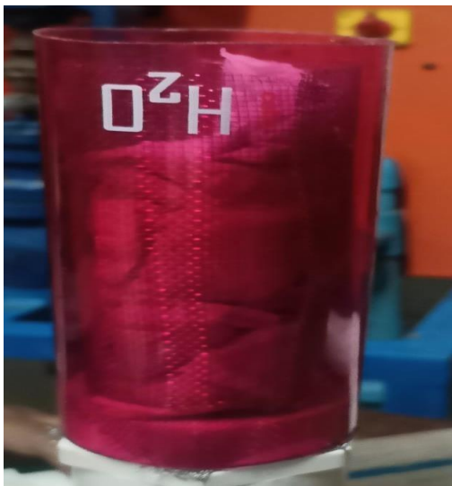
Fig.8. Waste PET bottle as Reactive Zone MOC
