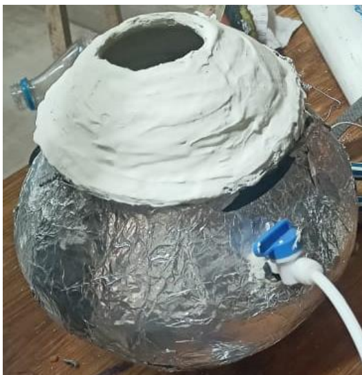
Fig 15 Earthen Pot with inbuilt heater for reboiler
