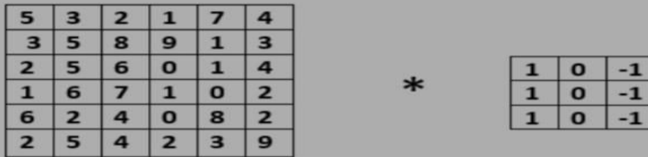
Figure 3. 6 \times 6 image with 3 \times 3 filter.
