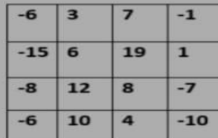
Figure 4. 4 \times 4 image after applying 3 \times 3 filter to 6 \times 6 image.
