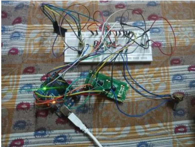
**Figure 3.1 Connections with Arduino, ESP8266, LCD, Potentiometer**
